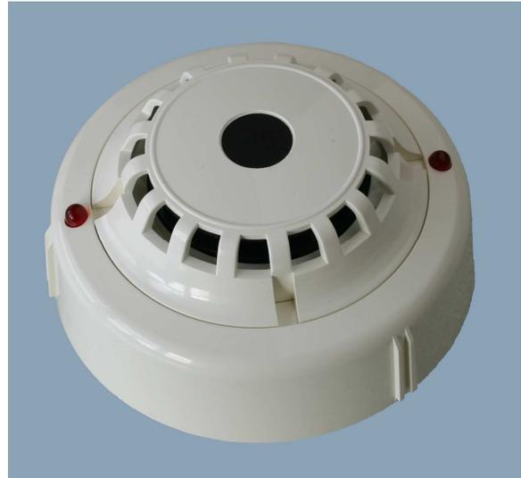
It responds to both visible and invisible smoke particles (aerosols) on the principle of detection of scattered infrared radiation.
