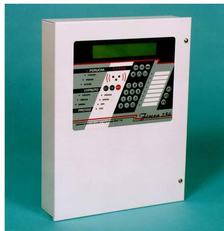
The analog addressable C.I.E. MHU 110 (MHU 111) is an equipment of the electric fire signalling that is intended to evaluate fire situations in the protected object. For operating the internal and external functions the C.I.E. makes use of the microprocessors Motorola - the first one is the general system microprocessor, the second one operates the lines with detectors.
