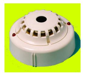
The MHG 231 detector is to install at places where occurrence and concentration of smoke is assumed. The detector is responsive to fouling – to both visible and invisible smoke particles (aerosols) – on the principles of detection of scattered infrared radiation.
