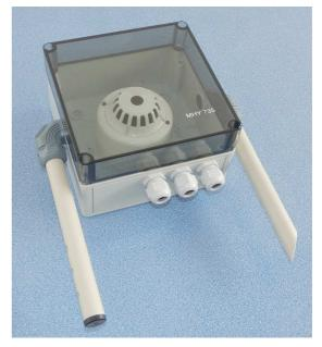
Adapter for air conditioning is a plastic box with transparent cover with 2 pipes through which air is carried inside the adapter.
