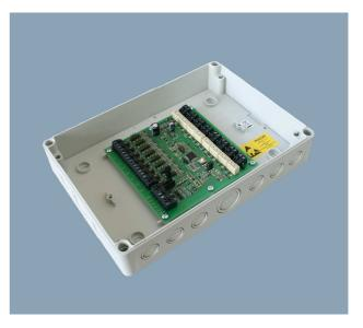
Inputs serve for automatic signalling of pre-defined exceptional states of any external device, which signals this state by either closing or opening an electronic contact, or by voltage applied to opto-isolated input. Inputs can also be set as monitored.
